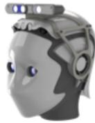
Fig. 2: Detail of the REEM head equipped with the depth sensor device.
